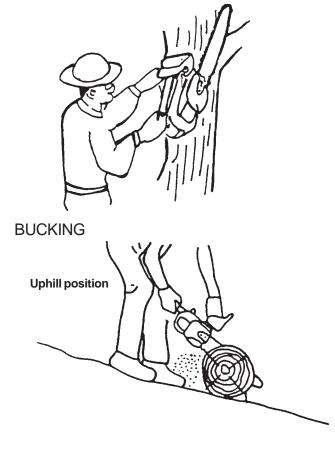
Don't cut with the saw overhead or the bar in a vertical position. If the saw should kick back you may not have good enough control to prevent possible injury.
